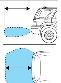
While receiving a warning the radio volume will be reduced to a predetermined level. After the warning goes away, the radio will return to the previous value. The RSS automatically turns on when the gearshift lever is placed in R (Reverse) and the ignition is on. A control in the message center allows the driver to disable the system, refer to *Message center* in the *Instrument Cluster* chapter for more information.
